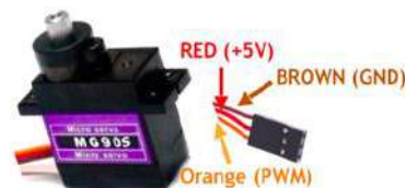
Figure 4. MG90S Servo Motor and Pinout
