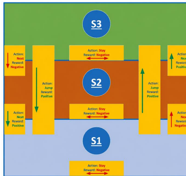
Figure 3. SARSA training environment illustrating state transitions (S1–S3), possible actions (stay, next, jump), and corresponding reward assignments
