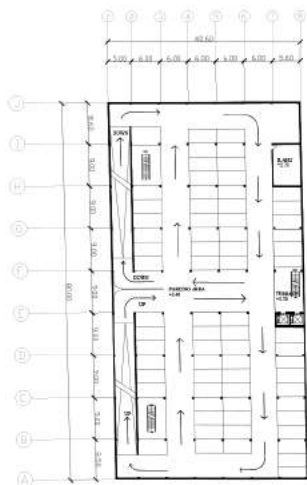
1ST FLOOR PARKING BUILDING SCALE 1:250
