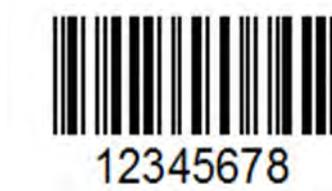
Gambar 4. Interleaved 2 of 5
